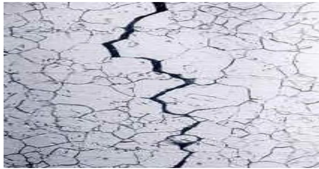
Figure 4: Stress Corrosion Cracking (from NACE)
