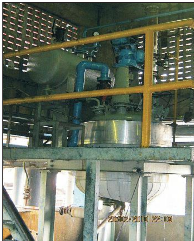
Main reactor in catalyst production unit at M/s Lona Industries Ltd., Mumbai
