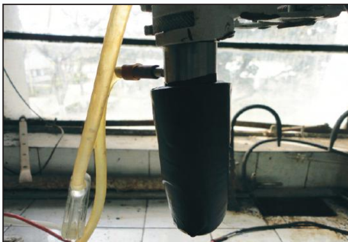
Determination of rate of wax deposition from crude oils by cold finger set-up
