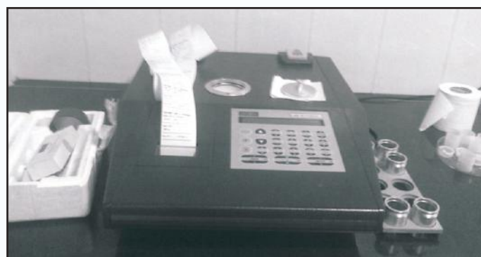
Oxford-XRF Sulphur Analyzer
