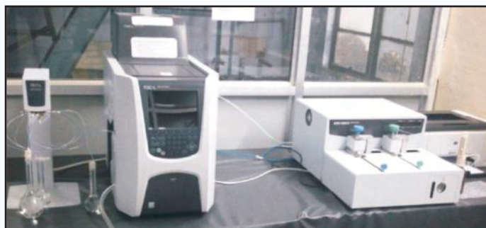
TOC instrument (Model: TOC-L CSH with TNML and SSM-5000A)
