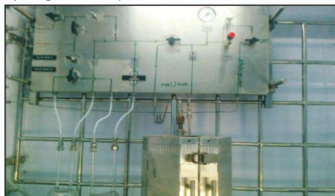
Catalyst Activation and Regeneration Reactor System
