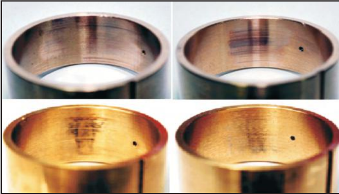
Worn-out bearing test specimens after experimentation
