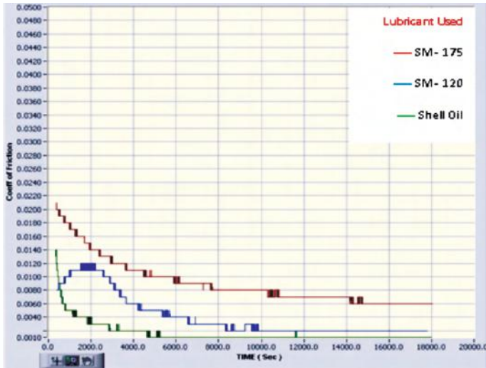
Friction behaviour of the gun metal bearings with different clearance and lubricants
