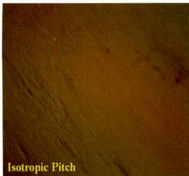
Figure : Optical micrograph of isotropic pitch
