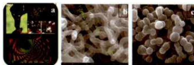
Figure 6: a) schematic diagram of project process b) SEM image of synthesized carbon nano tube c) SEM image of carbon nano-granules
