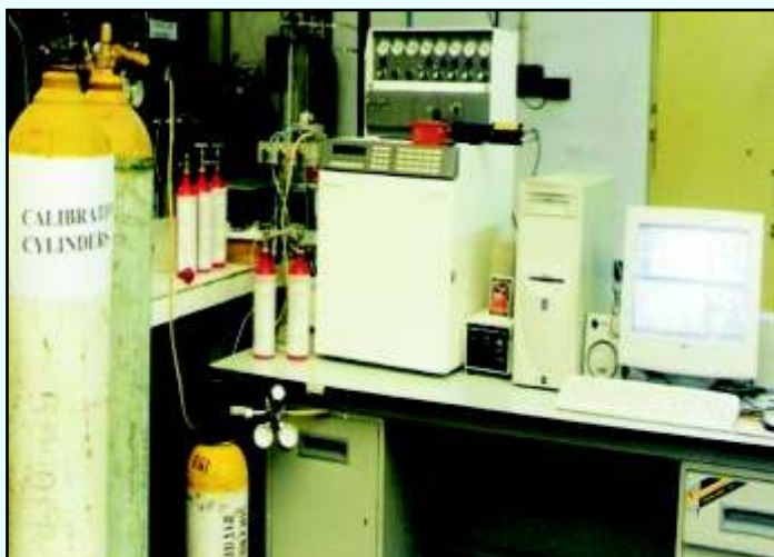
GC facility for analyzing gas streams
