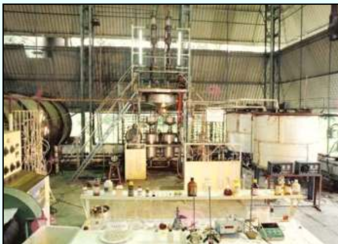
Pilot plant for gas desulphurization studies
