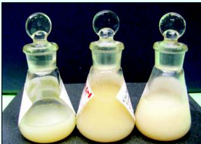
FT synthesis paraffin wax obtained from syn gas
