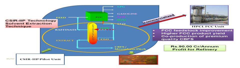
A technology for producing additional quantity of clean feed (low sulfur and aromatics) for Fluid Catalytic Cracking (FCC) unit and premium quality Carbon Black Feed Stock (CBFS) simultaneously from low value petroleum refinery stream
